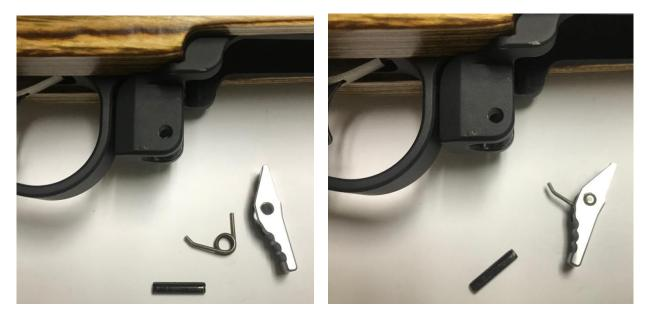
Align the spring, magazine latch and slave pin with the hole in the floor plate and using a non-marring punch or hammer, drive the roll pin to push out the slave pin and engage with both sides of the floor plate latch mount.
